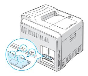
8 Insert the ends of the memory DIMM into the slots on the levers.
